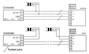
Controller with 3-wire connection
