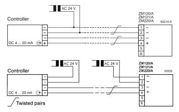
Note: Several DC 4 ... 20 mA receivers can be driven by the same control signal (series connection – check input impedance!).
