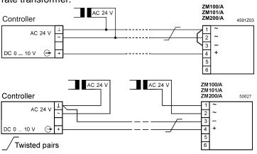
Note: If, for reasons of cross-section, the AC 24 V and DC 0 ...10 V (or DC 4 ... 20 mA) cables are routed separately, the AC 24 V cable need not be twisted.
