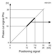
Typical operating range of valves with magnetic actuators (0...100 % stroke).
