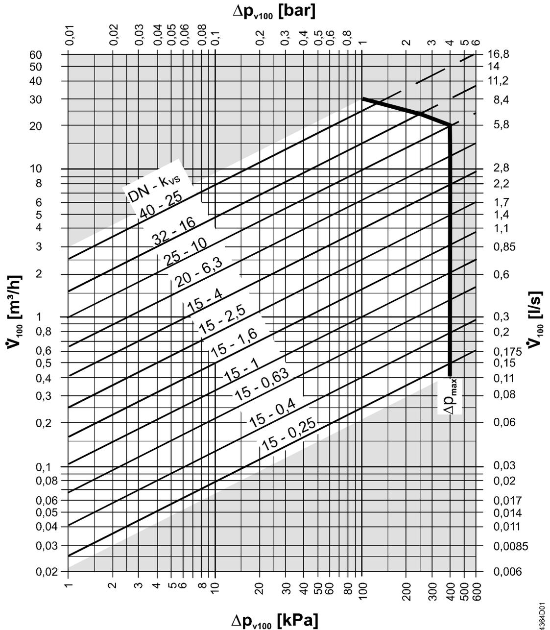
$\Delta p_{max}$  = Maximum permissible differential pressure across the valve (VXG44...: mixing port: Ports A-AB, B-AB, diverting: Ports AB-A, AB-B), valid for the entire actuating range valve-actuator unit
