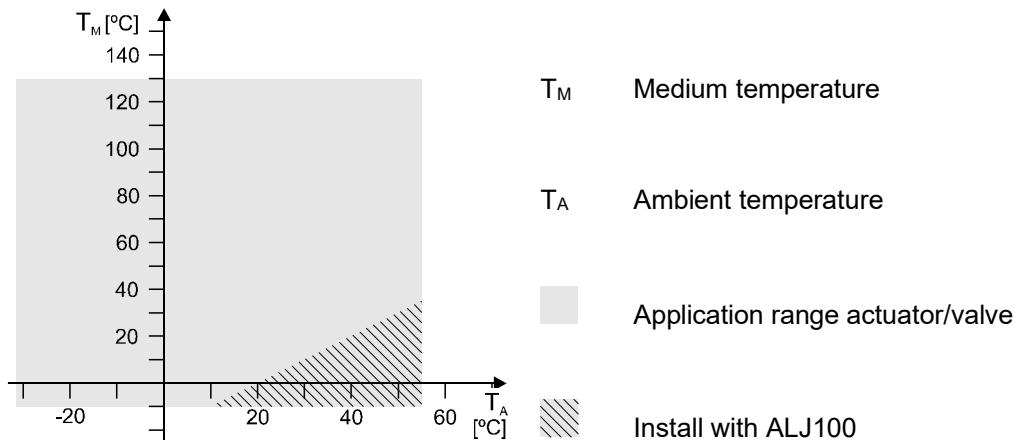
Only use GDB.., GDD.., GSD.. and GQD.. actuators at medium temperatures  $> 0$  °C.
