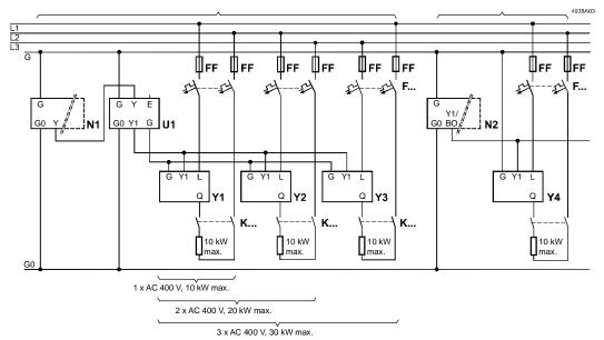
Connection diagram 3 (standard circuit)
