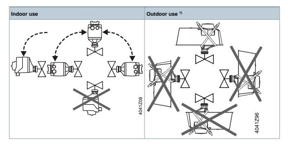
1) Requires the weather shield ASK39.2 Degree of protection of housing IP54 remains unchanged.
