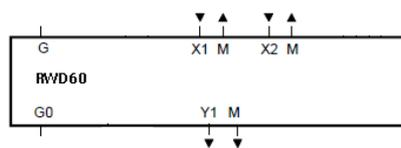
⚠ Power supply ground (G0) is internally connected to signal ground (M).
