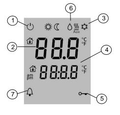
2. Display room temperature, setpoints and control parameters.
