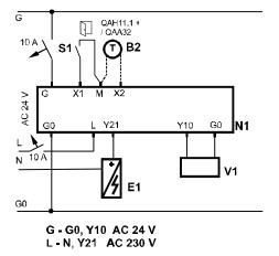
VAV / CAV system, V1 DC 0...10V actuator for heating or cooling
