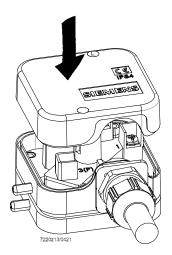
Step 11: Screw tight the cover (maximum torque 1 Nm)
