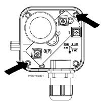
Step 5: Loosen the M20 cable gland
