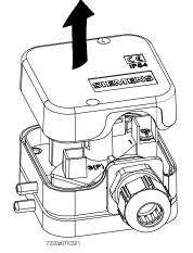
**Step 4:** Screw on the pressure switch diagonally with at least 2 screws. 4 screws must be used for degree of protection IP54. Use suitable M4 screws (maximum torque 1 Nm) or comparable screws for fastening
