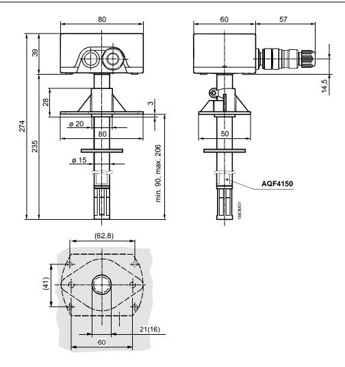
Drilling template with (without) mounting flange
