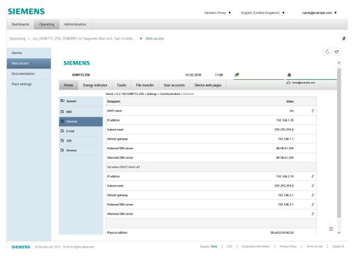
Click the symbol do to open the web server user interface under a new tab and is then the same as the view under a direct connection.
