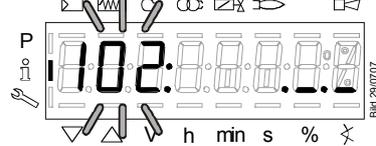
The display shows parameter **102**: flashing on the left, characters **.\_.** on the right.
