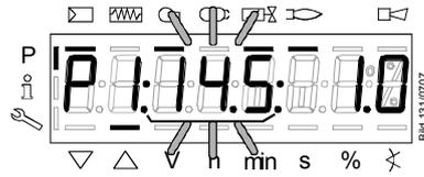
Keep **F** depressed and press **-** or **+** to adjust the fuel actuator.
