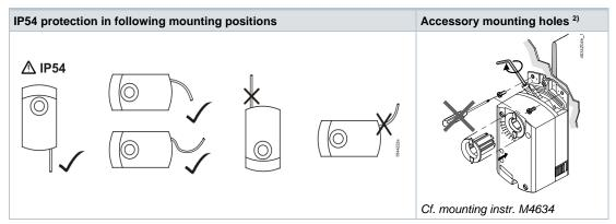
Not to be used for fixation of the actuator, use anti-rotation-bracket instead.
