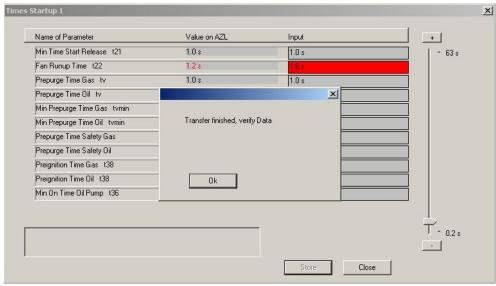
Fig. 14: Fault during the parameter setting procedure
