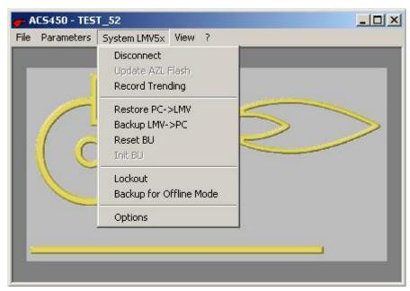
Fig. 20: Resetting/initializing the basic unit
