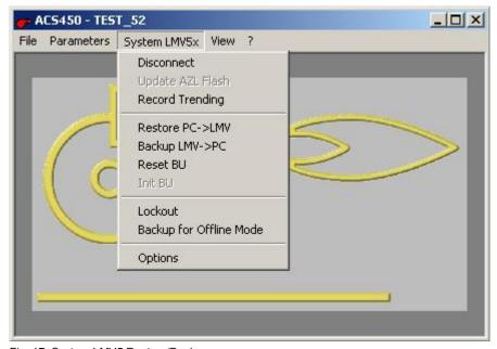
Fig. 17: System LMV5 Restore/Backup
