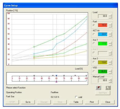
Fig. 24: Setting elements for the manual load
