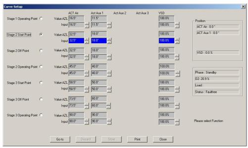
Fig. 28: Dialog for multistage fuel/air ratio control
