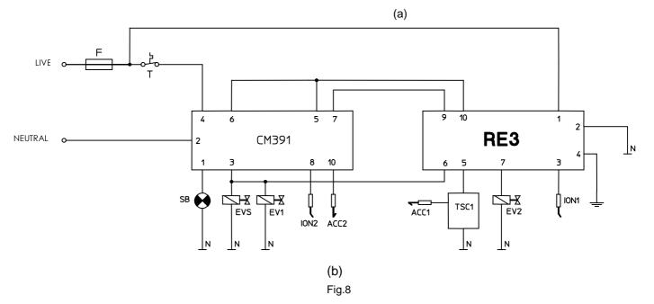
The diagram in Fig.8a differs from the one in Fig.8b for the presence of fan control and air pressure switch. This connection permits the ignition of two burners in sequence, with cross checking of the "flame on" state. A contact of the internal relay of RE3 is used to check the efficiency of the detector to prevent the beginning of the ignition cycle if the detector doesn't operate correctly.
