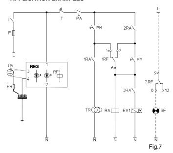
By releasing the button PM, the ignition transformer is turned off and the operation continues until one of the following situations occurs:
