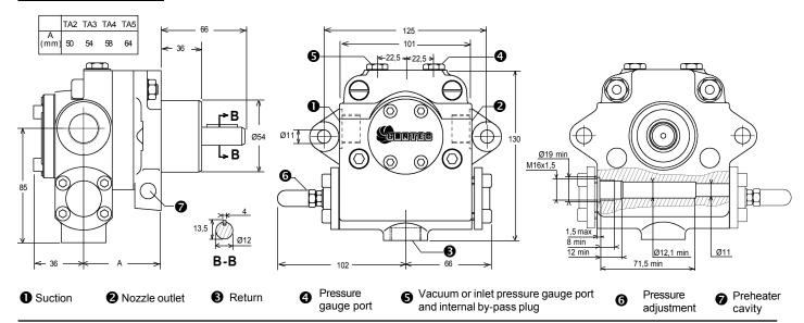
Example shows "C" rotation - Reverse all pump connections for "A" rotation.
