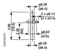
Figure 6. Duct Adapter Dimensions.
