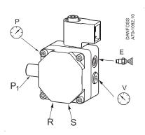
Note! Shaft rotation, location of nozzle outlet and other connections are seen from shaft end.
