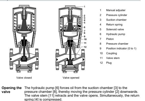
**Closing the** Activating the solenoid valve [5] allows the oil in the pressure chamber to flow back into the suction chamber. The compressed return spring moves the pressure cylinder upwards. The valve stem extends and the valve closes.
